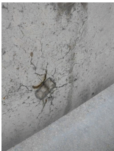
Fig. 8 Visual aspect of element E2 after 22 years exposure. Generally, still without any significant damages. Some minor cracks attributed to how the walls were cast.
