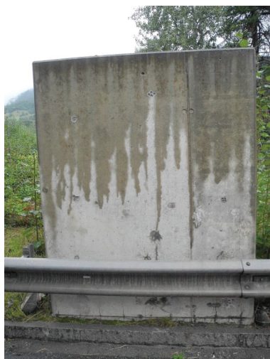
Fig. 8 Visual aspect of element E2 after 22 years exposure. Generally, still without any significant damages. Some minor cracks attributed to how the walls were cast.
