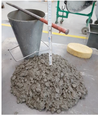
Figure 7. Slump test with Abram's cone on RM concrete
