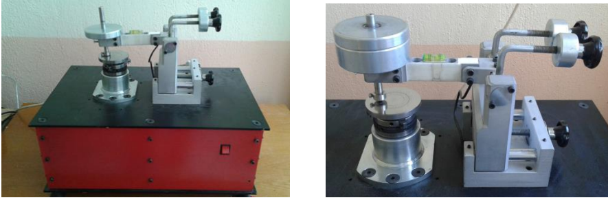
Fig. Pin on disc type wear test machine.
