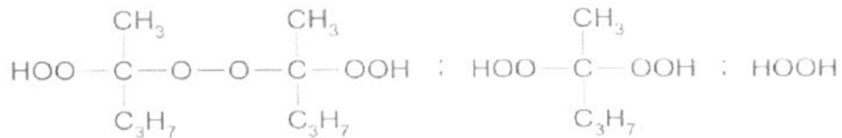
Figure 3: Structure of Methyl isopropyl ketone peroxide in dimethyl phthalate
